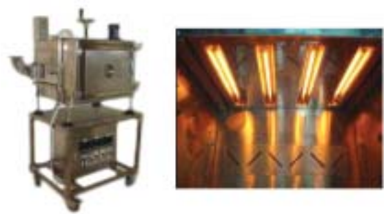
Fig. 2 Business oven model of microwave combined with infrared heat source
