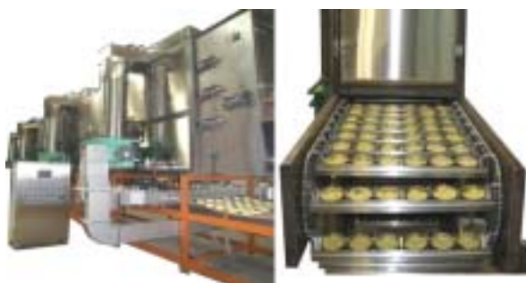
Fig. 1 Commercial experimental machine of microwave-assisted hot air dryer for non-fried instant noodles
