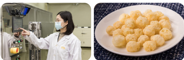
▲ Microwave vacuum equipment (left) and puffed cheese (right).
