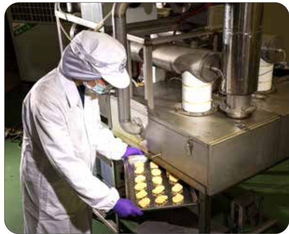
Superheated steam impingement flow-assisted frying equipment.
