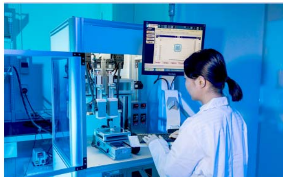
Trial production of plant protein products using food 3D printing technology
