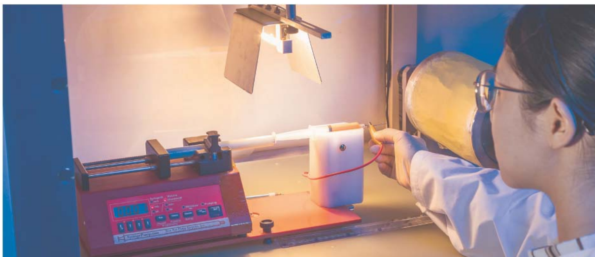
Coating with protein fibers using food electrospinning technology
