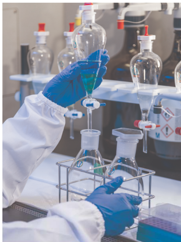
Sample pretreatment for pesticide and veterinary drug residues testing
