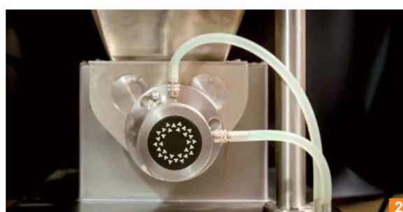
A semi-continuous process of simple shear operation for anisotropic structure of meat analogues
