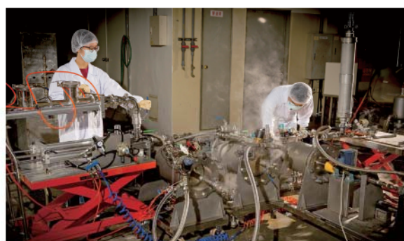
A semi-continuous process of simple shear operation for anisotropic structure of meat analogues
