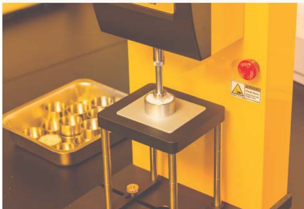
Application of texture analyzer on texture grading assessment of rice
