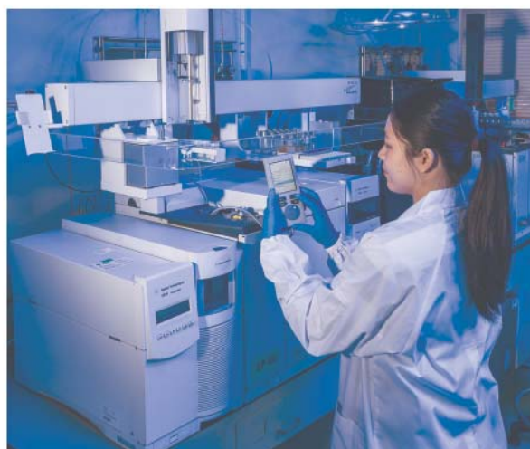
Analyses of volatile compounds using GC-MS combined with Multifunction Injector
