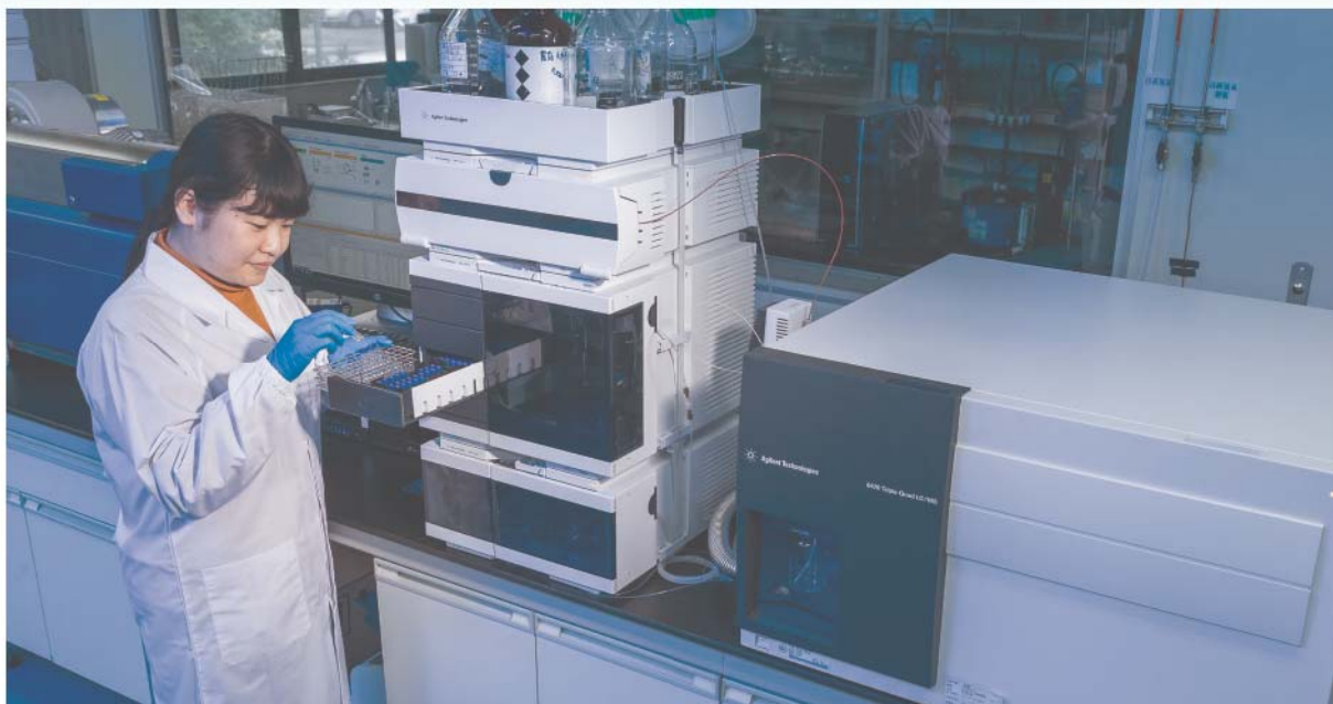
GC/MS/MS-for hazardous substance analysis – pesticide residues, veterinary drug residues and others
